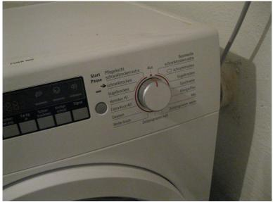
5) If finished set to Aus, empty dust filter and water tank.
